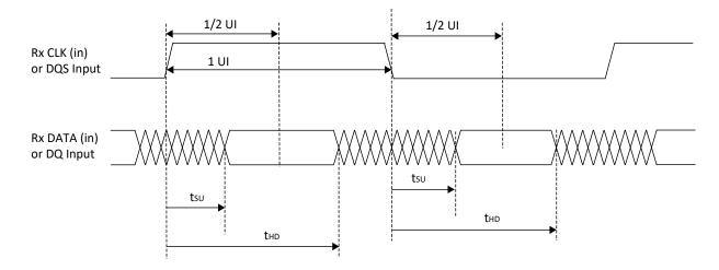
Figure 3.8. Receiver RX.CLK.Aligned and DDR Memory Input Waveforms
