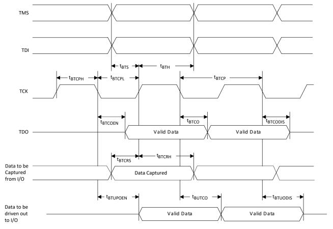
Figure 3.23. JTAG Port Timing Waveforms
