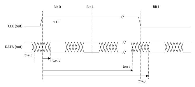
Figure 3.13. Transmitter DDRX71\_TX Waveforms
