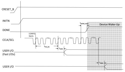
Figure 3.22. Slave SPI/I<sup>2</sup>C/I3C Wake-Up Timing
