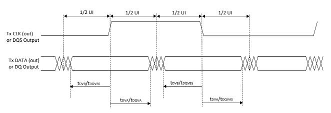
Figure 3.9. Transmit TX.CLK.Centered and DDR Memory Output Waveforms
