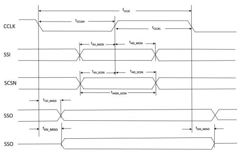
Figure 3.19. Slave SPI Configuration Timing
