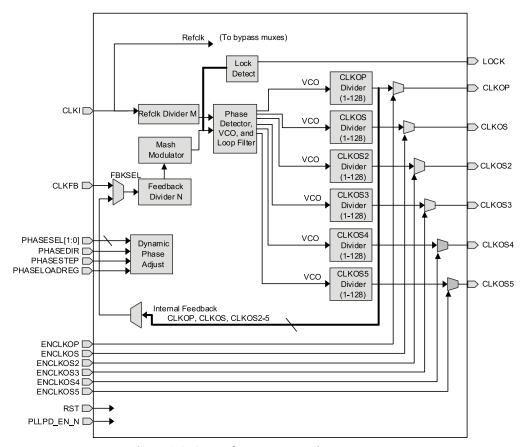
Figure 2.6. General Purpose PLL Diagram
