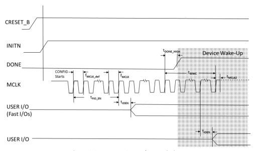
Figure 3.21. Master SPI Wake-Up Timing
