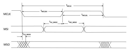
Figure 3.18. Master SPI Configuration Timing
