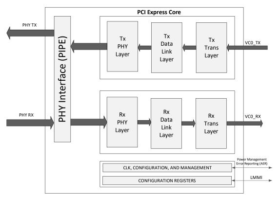
Figure 2.28. PCIe Core
