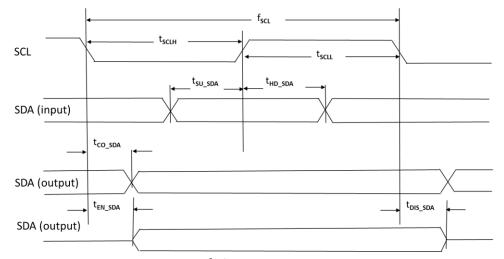
Figure 3.20. I<sup>2</sup>C/I3C Configuration Timing
