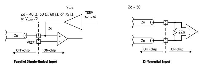
Figure 3.1. On-Chip Termination
