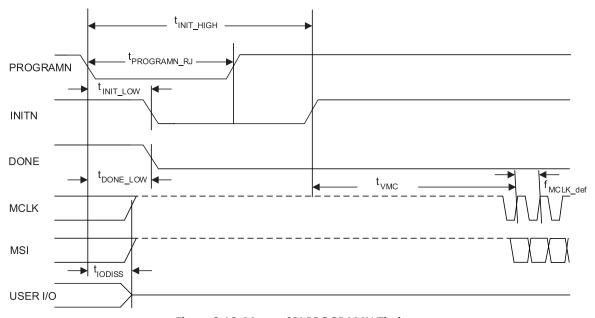
Figure 3.16. Master SPI PROGRAMN Timing
