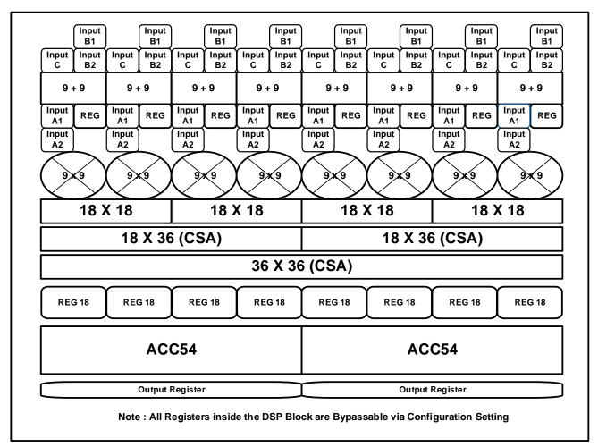
Figure 2.16. Certus-NX DSP Functional Block Diagram
