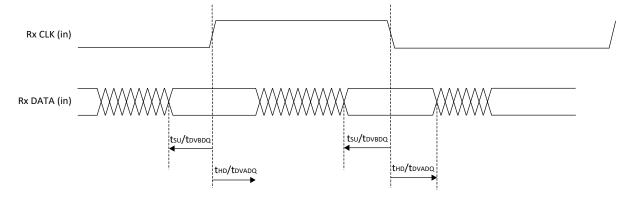
Figure 3.7. Receiver RX.CLK.Centered Waveforms
