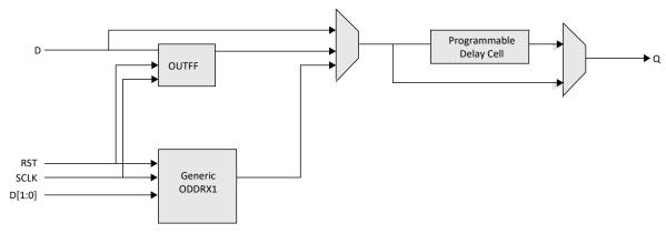
Figure 2.21. Output Register Block on Top, Left, and Right Sides
