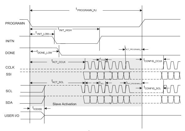
Figure 3.17. Slave SPI/I<sup>2</sup>C/I3C PROGRAMN Timing
