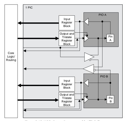
Figure 2.18. Wide Range Programmable I/O Cells
