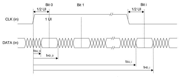
Figure 3.12. Receiver DDRX71\_RX Waveforms
