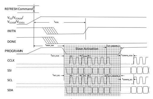
Figure 3.15. Slave SPI/I<sup>2</sup>C/I3C POR/REFRESH Timing
