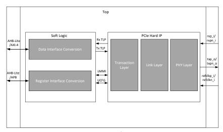
Figure 2.29. PCIe Soft IP Wrapper
