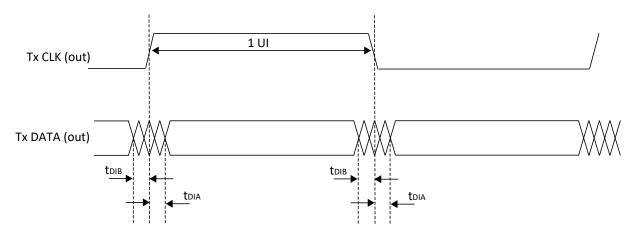
Figure 3.10. Transmit TX.CLK.Aligned Waveforms
