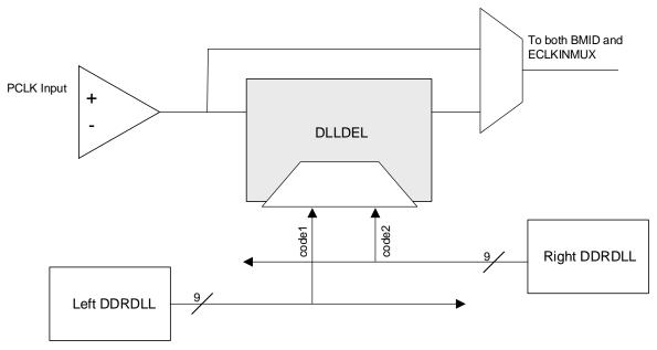
Figure 2.11. DLLDEL Functional Diagram
