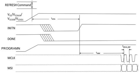
Figure 3.14. Master SPI POR/REFRESH Timing
